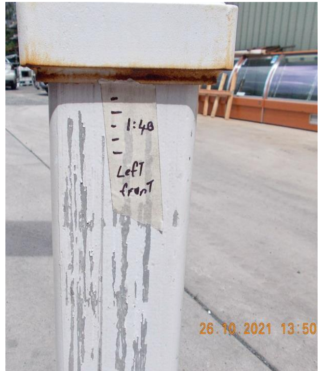
Fig 10. The The left front outrigger - Creep testing
