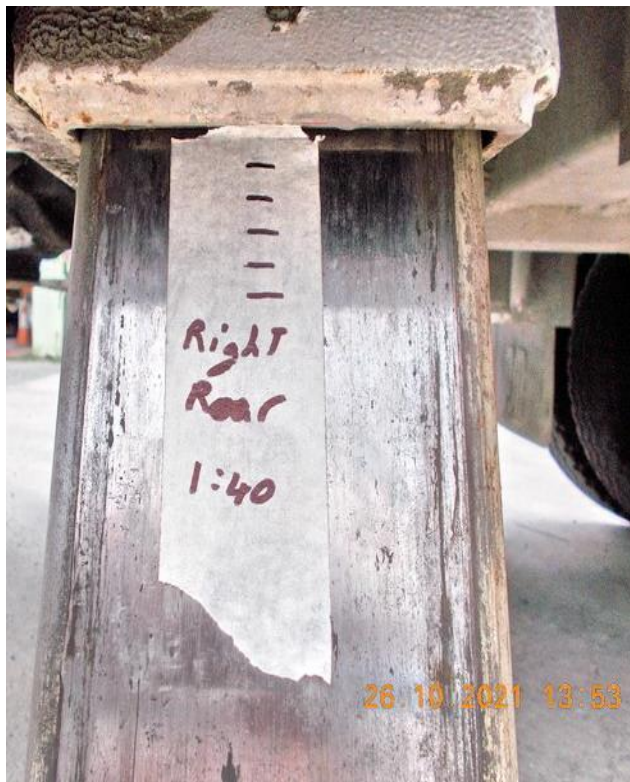
Fig 11. The right rear outrigger - Creep testing
