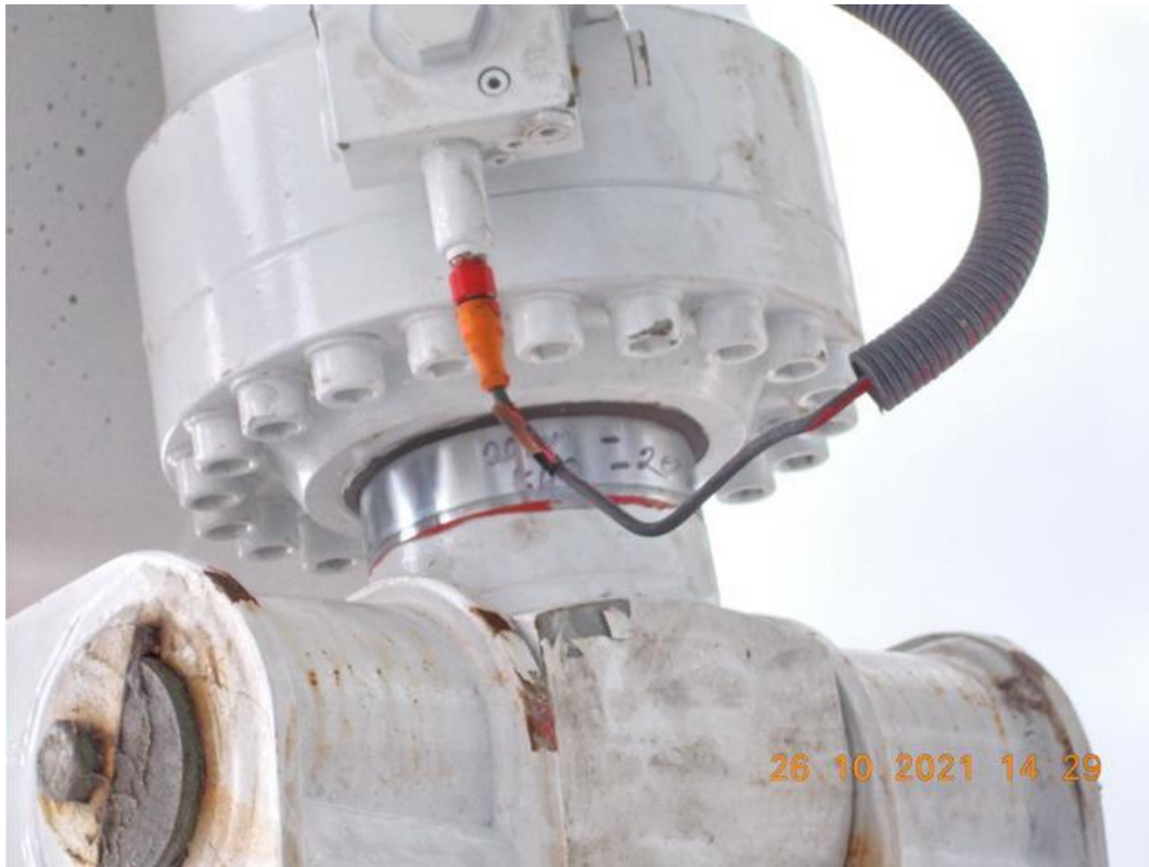
Fig 5. The first boom cylinder - Creep testing
