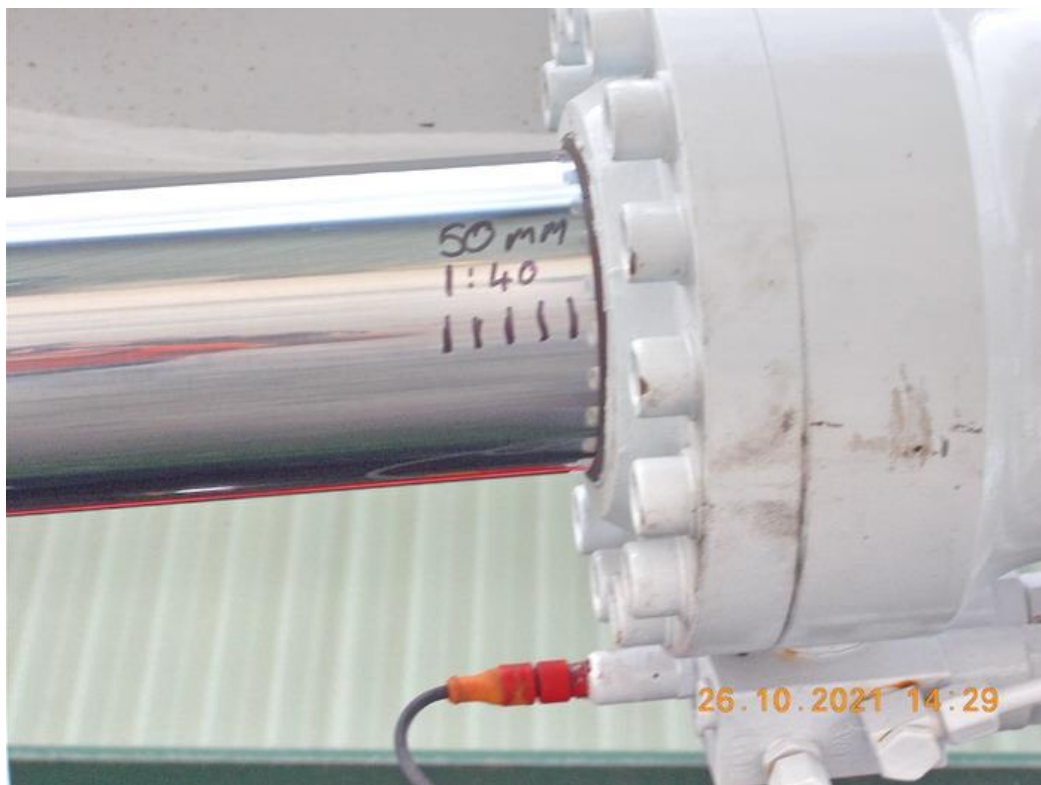
Fig 6. The second boom cylinder - Creep testing
