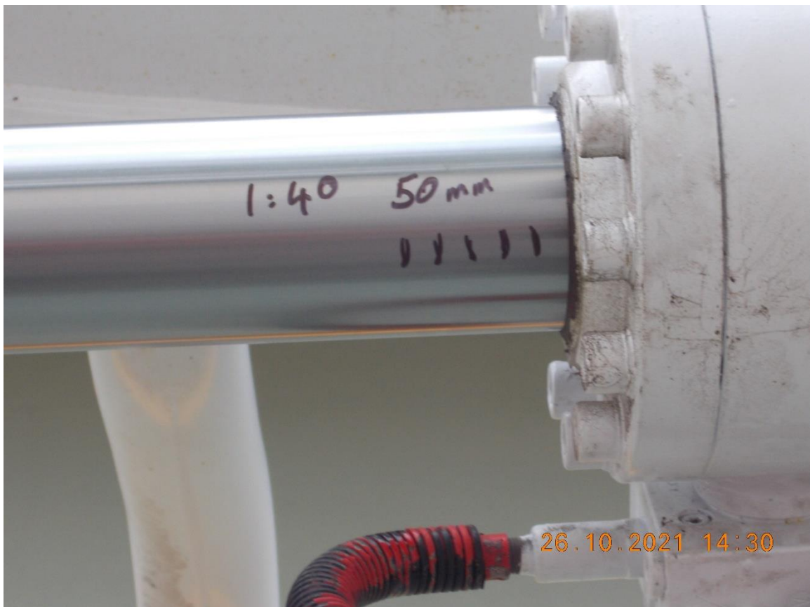
Fig 8. The fourth boom cylinder - Creep testing
