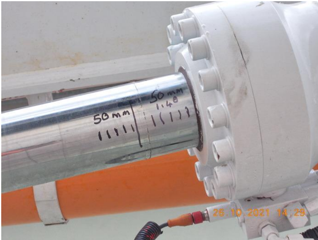
Fig 7. The third boom cylinder - Creep testing
