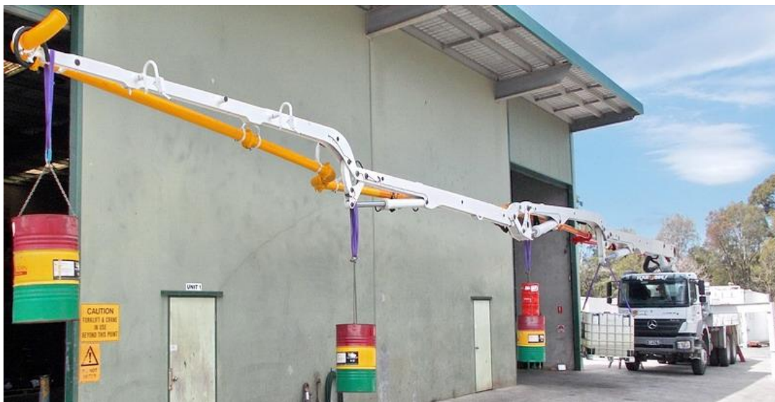
Fig 2. Load testing of the boom – Day 2
