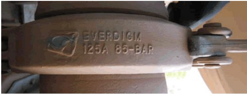
Figure 2. An example of acceptable marking on pipe clamps.
